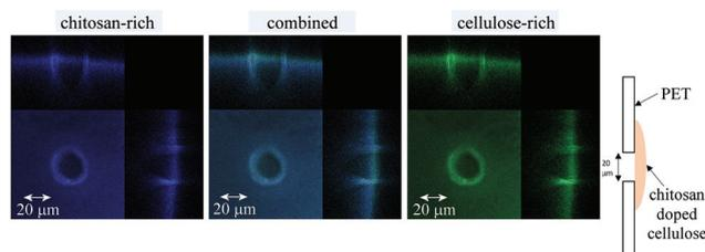
Fig. 4 Fluorescence images in top view and side view for the cellulose fluorescence (left, blue), the chitosan fluorescence (right, green), and the combined cellulose and chitosan fluorescence (middle, blue and green). A schematic drawing is shown to allow the features to be identified.
