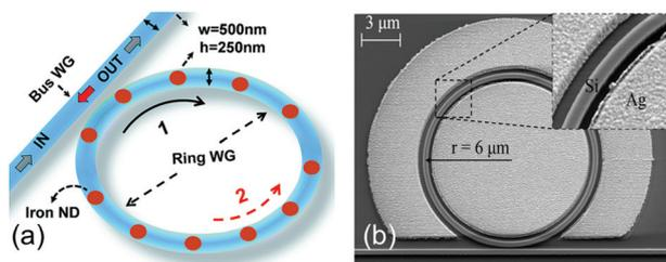
**Fig. 10** Hybrid WGM structures for bulk refractive index sensing. (a) SOI ring resonator decorated with metallic nanodisks along the circumference. Reproduced from ref. 89 with permission from The Royal Society of Chemistry. (b) Metal–dielectric double slot SOI ring resonator. The inset shows the gap between the silicon ring and the surrounding silver plate, which is the region of accumulation of the electromagnetic field. Reproduced from ref. 94.
