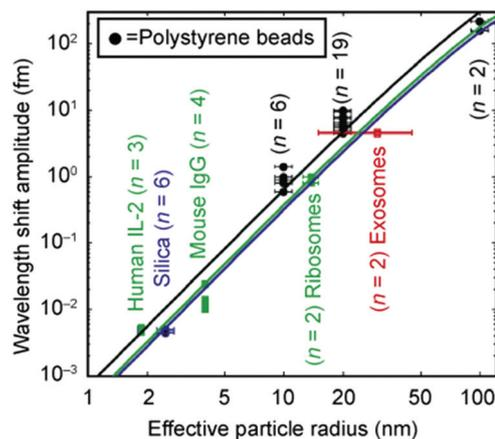
**Fig. 12** State of the art for single particle detection using a purely photonic WGM resonator. Wavelength shift as a function of the particle radius for different types of synthetic and biological nanoparticles: human interleukin-2 molecules, SiO<sub>2</sub> beads, mouse immunoglobulin, human ribosomes, mouse exosomes, and polystyrene nanobeads. The solid lines are calculated from the reactive sensing principle (eqn (6)). Reproduced from ref. 121.
