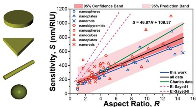
Fig. 6 Bulk sensitivity (in units of  $\text{nm RIU}^{-1}$ ) of different types of plasmonic nanostructures supporting LSP resonances with different aspect ratios. Different symbols correspond to different structures. Reproduced with permission from A. U. Khan *et al.*, *J. Phys. Chem. C*, 2016, **120**, 19353–19364 (ref. 59). Copyright 2016 American Chemical Society. For the meaning of the different colours, lines and shades the reader is referred to ref. 59.
