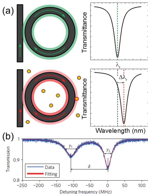
**Fig. 3** (a) Graphical illustration of the reactive sensing principle. The resonance of the unperturbed cavity (upper panels) redshifts after the binding of a nanoparticle (bottom panels). (b) Resonance splitting induced by a single nanoparticle bound to a high  $Q$ -factor toroidal micro-resonator. Reproduced from ref. 28.
