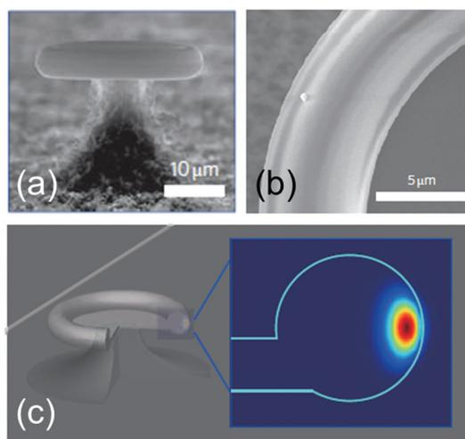
**Fig. 11** Single particle detection with a purely photonic WGM resonator. (a) SEM image of a micro-toroid (diameter: 40  $\mu\text{m}$ ) used for the optical measurement. (b) SEM detail of a PS nanoparticle (diameter: 300 nm) bound to the surface of the toroid. (c) 3D rendering of the micro-toroid employed in the numerical simulations and cross section of the electric field of the WGM mode. Reproduced and adapted from ref. 28.
