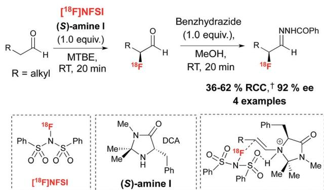
Scheme 5 Chiral imidazolidinone (*S*)-I for the enantioselective  $^{18}\text{F}$ -fluorination of aldehydes with  $^{18}\text{F}$ -NFSI.  $\dagger$ RCC determined by radio-HPLC relative to  $^{18}\text{F}$ -NFSI. DCA = dichloroacetic acid. For  $^{18}\text{F}$ -NFSI, SA =  $0.05 \text{ Ci } \mu\text{mol}^{-1}$ , ( $n = 3$ ).
