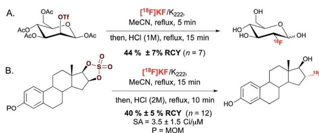
Scheme 1 (A.) Radiosynthesis of 2- $[^{18}\text{F}]$ fluoro-2-deoxy-D-glucose ( $[^{18}\text{F}]$ FDG). (B.) Radiosynthesis of 16- $\alpha$ - $[^{18}\text{F}]$ fluoroestradiol ( $[^{18}\text{F}]$ FES). SA = specific activity. MOM = methoxymethyl.
