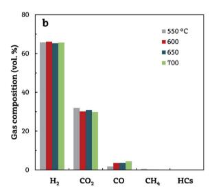
Fig. 3 Effect of reforming temperature on the yields of the gaseous products (a) and their concentrations (on a dry basis) (b). Reforming conditions: space time, 20  $g_{cat}$  min  $g_{volatiles}^{-1}$ , S/B ratio, 4.
