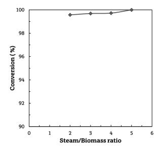
Fig. 6 Effect of S/B ratio on conversion. Reforming conditions:  $600\,^{\circ}\text{C}$ ; space time,  $20\,\,\text{g}_{\text{cat}}$  min  $\text{g}_{\text{volatiles}}^{-1}$ .
