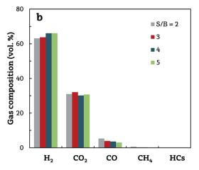
Fig. 7 Effect of S/B ratio on the yields of the gaseous products (a) and their concentrations (on a dry basis) (b). Reforming conditions:  $600\,^{\circ}\text{C}$ ; space time,  $20\,_{\text{gat}}$  min  $g_{\text{volatiles}}^{-1}$ .
