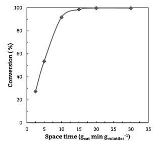
Fig. 4 Effect of reforming space time on conversion. Reforming conditions:  $600\,^{\circ}\text{C}$ ; S/B ratio, 4.
