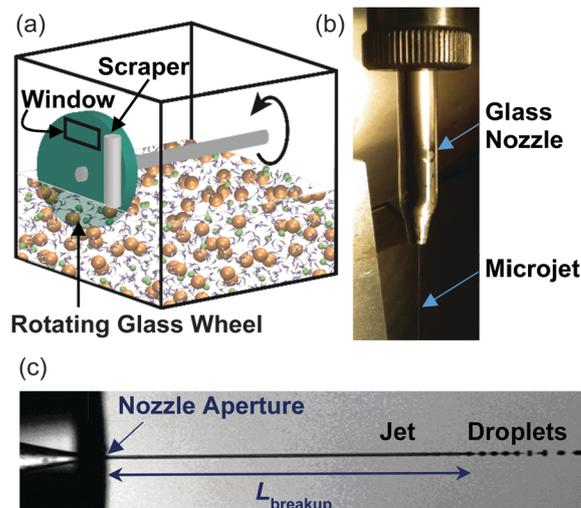
**Fig. 2** Two methods for generating continuously renewed liquids in vacuum. (a) A rotating glass wheel picks up a thin film of liquid, shown here as salty water, which is scraped to a uniform thickness. (b) Liquid microjets are created by pressurizing liquid through a glass nozzle. (c) The cylindrical microjet breaks up into droplets a distance  $L_{\text{breakup}}$  away from the nozzle orifice. Photos provided by Diane Lancaster and Manfred Faubel.
