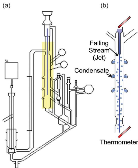
**Fig. 1** (a) Hickman's falling-stream tensimeter apparatus designed in 1952 to measure evaporation coefficients. (b) Close-up view of the falling stream and condensate collection ports. Adapted with permission from K. C. D. Hickman and D. J. Trevoy, *Ind. Eng. Chem.*, 1952, **44**, 1882–1888. Copyright 1952 American Chemical Society.
