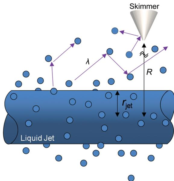
Fig. 4 Evaporating molecules create a vapor cloud surrounding the liquid microjet. The number of vapor–vapor collisions over the distance  $R$  depends on both the mean free path  $\lambda$  and the jet radius  $r_{\text{jet}}$ .
