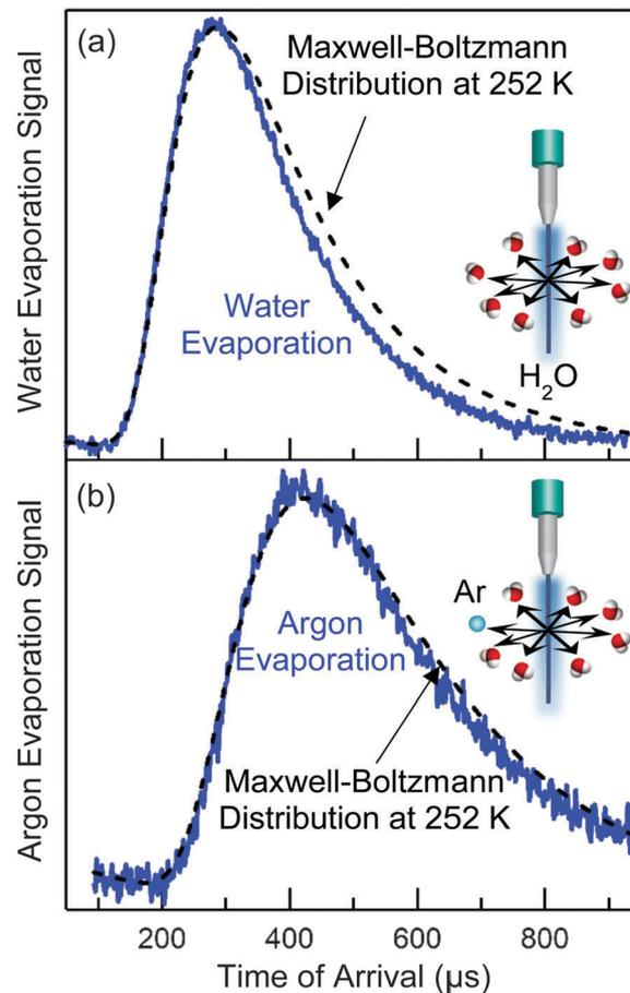
Fig. 5 Time-of-flight (TOF) spectra of (a) water molecules and (b) dissolved argon atoms evaporating from a pure water microjet of radius  $r_{\text{jet}} = 5 \mu\text{m}$ . The best-fit dashed lines are Maxwell–Boltzmann distributions at  $T_{\text{liq}} = 252 \text{ K}$ . Adapted with permission from C. Hahn, Z. R. Kann, J. A. Faust, J. L. Skinner and G. M. Nathanson, *J. Chem. Phys.*, 2016, **144**, 044707. Copyright 2016, AIP Publishing LLC.
