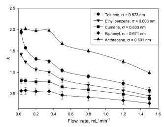
Fig. 1 Influence of the mobile phase flow rate on the retention factors for model compounds on the UiO-66@SiO $_2$  column. Mobile phase – n-hexane, 25 °C, sample volume 2  $\mu$ L of 100  $\mu$ g mL $^{-1}$  solutes in n-hexane. Kinetic diameter ( $\sigma$ , nm) for each analyte was calculated as suggested by Jae et  $al.^{16}$  using critical constants from. $^{17}$
