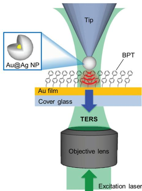
**Fig. 3** Measurement of TERS. The monolayer of biphenyl-4-thiol (BPT) is self-assembled on an Au coated cover glass. Laser beam is focused on the Au@Ag NP attached tip through an objective lens and the Raman radiation is collected through the same objective lens.
