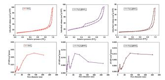
Fig. 4 The nitrogen adsorption–desorption isotherms and pore size distributions of as-prepared MnO<sub>2</sub>, Fe<sub>3</sub>O<sub>4</sub>@MnO<sub>2</sub> and Fe<sub>2</sub>O<sub>3</sub>@MnO<sub>2</sub> nanocomposites samples at time of 6 h calculated by BJH method.
