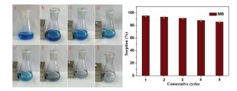
Fig. 7 Regeneration studies of as-prepared Fe<sub>3</sub>O<sub>4</sub>@MnO<sub>2</sub> nanocomposites in the removal of MB. The photographs showed the MB solution (a) and adsorption process under magnetic separation at different time intervals ((b)-(h) 0, 10, 20, 30, 40, 50, and 60 min).
