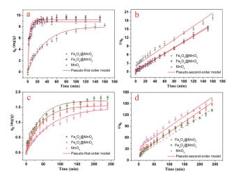
Fig. 6 Adsorption kinetics curves of as-prepared Fe<sub>3</sub>O<sub>4</sub>@MnO<sub>2</sub> and Fe<sub>2</sub>O<sub>3</sub>@MnO<sub>2</sub> nanocomposites onto MB (a and b) and RhB (c and d) at 298 K.
