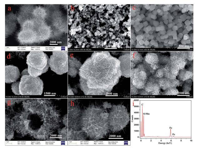
Fig. 1 SEM images of as-prepared nanostructures. (a) MnO<sub>2</sub>; (b) Fe<sub>3</sub>O<sub>4</sub>; (c) Fe<sub>2</sub>O<sub>3</sub>; (d)-(g) Fe<sub>3</sub>O<sub>4</sub>@MnO<sub>2</sub> prepared at times of 3 h, 6 h, 9 h, and 15 h, respectively; (h) Fe<sub>2</sub>O<sub>3</sub>@MnO<sub>2</sub> prepared at time of 6 h; (i) typical EDXS of Fe<sub>3</sub>O<sub>4</sub>@MnO<sub>2</sub> nanocomposites prepared at 6 h.
