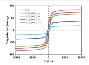
Fig. 5 Hysteresis loops of as-prepared  $Fe_3O_4$  nanoparticle and  $Fe_3O_4$ @MnO<sub>2</sub> nanocomposites at different time intervals at 298 K.
