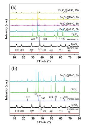
Fig. 3 XRD patterns of as-prepared MnO<sub>2</sub>, Fe<sub>3</sub>O<sub>4</sub>@MnO<sub>2</sub> (a) and Fe<sub>2</sub>O<sub>3</sub>@MnO<sub>2</sub> (b) nanocomposites.
