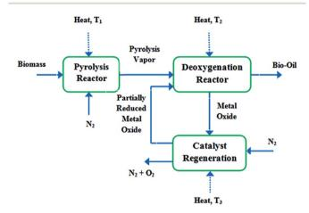
Fig. 8 Schematic of the chemical looping deoxygenation (over metal oxide catalysts) concept  $(T_3 > T_1 > T_2)$ .<sup>103</sup>
