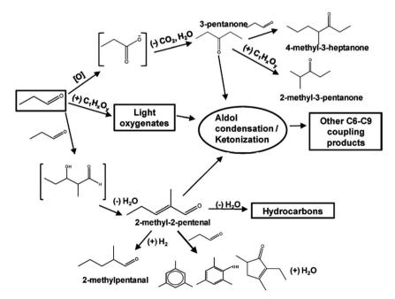
Fig. 7 Proposed reaction mechanism for propanal conversion over Ce<sub>0.5</sub>Z<sub>0.5</sub>O<sub>2</sub> – adapted from Gangadharan et al. 102
