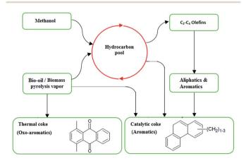
Fig. 10 Kinetic scheme suggested for the bio-oil/biomass and methanol mixture conversion into hydrocarbons and coke on HZSM-5 catalysts. Adapted from Valle et al. 115
