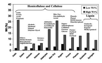
Fig. 1 Bio-oils (derived from lignocellulosic biomass) chemical composition.  $^{30}$
