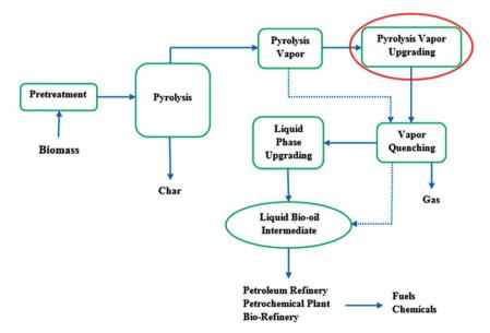
Fig. 2 Schematic of pyrolyis process and upgrading – highlighting pyrolysis vapor upgrading
