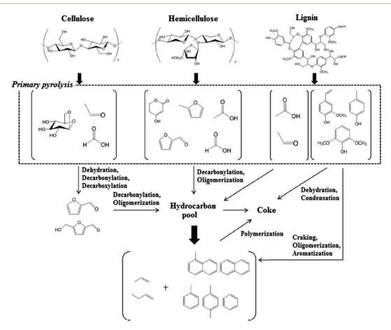
Fig. 3 Reaction pathways for pyrolysis and catalytic pyrolysis vapor upgrading of lignocellulosic biomass over HZSM-5 catalyst. Adapted from Wang et al.<sup>70</sup>
