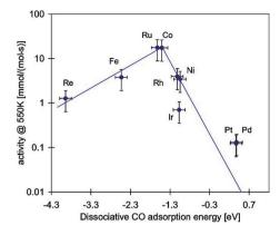
Fig. 3 Activities of different supported transition metal catalysts as a function of the reaction energy for dissociative carbon monoxide chemisorption. Reprinted from ref. 26, Copyright (2004), with permission from Elsevier.
