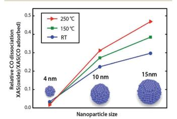
Fig. 10 Relative concentrations of dissociated CO species on 4, 10, and 15 nm nanoparticles after exposure to CO/He at different temperatures. Reproduced with permission from ref. 114 Copyright (2013) American Chemical Society.
