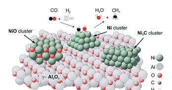
Fig. 4 Sketch of the catalyst structure and selective reactions occurring during the synthesis of methane. Reprinted from ref. 75, Copyright (2007), with permission from Elsevier.
