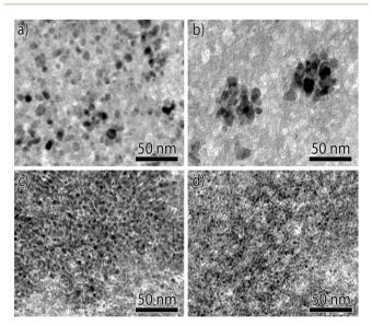
Fig. 7 Bright-field TEM images of Ni/SiO $_2$  catalysts with different Ni particle sizes after reduction: (a)  $\sim$ 8 nm, (b)  $\sim$ 9 nm, (c)  $\sim$ 4 nm, and (d)  $\sim$ 3 nm. Reproduced with permission from ref. 66 Copyright (c) [2014 WILEY-VCH Verlag GmbH & Co. KGaA, Weinheim].
