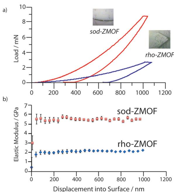
Fig. 2 Representative (a) load vs. displacement curves and (b) elastic moduli values as a function of depth for **1** and **2**. Error bars are taken from the standard deviation of more than 15 indents.
