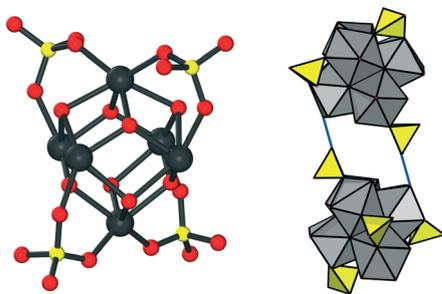
Fig. 4 Left: the core architecture of the inorganic node in 2. Zirconium atoms are shown in black, oxygen atoms in red and sulphur atoms in yellow. Right: two inorganic nodes interacting *via* hydrogen bonds. ZrO polyhedra are shown in grey, sulfate ions in yellow and hydrogen bonds as blue lines.
