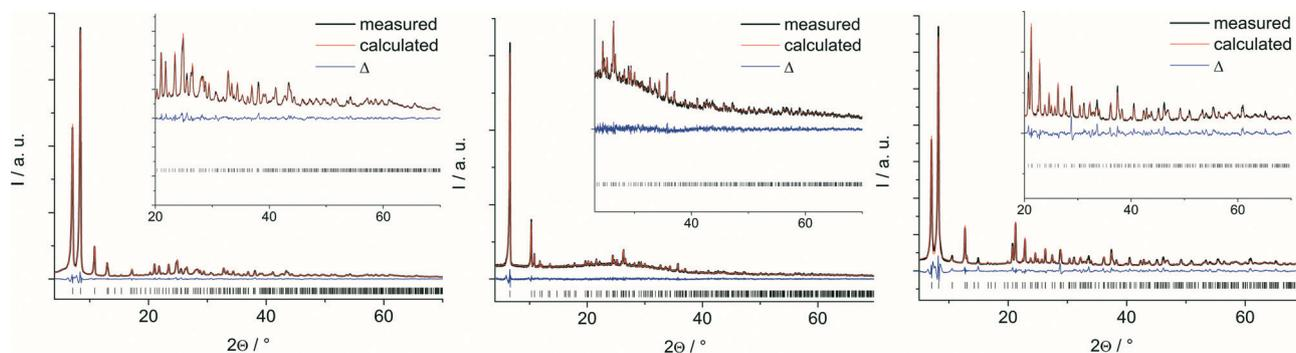
**Fig. 2** Final plots of the Rietveld refinements of **1**, **2** and **3** (from left to right). Measured data are shown as black lines and calculated fit as red lines; the blue curves indicate the difference plots. Vertical bars mark the allowed Bragg reflection positions
