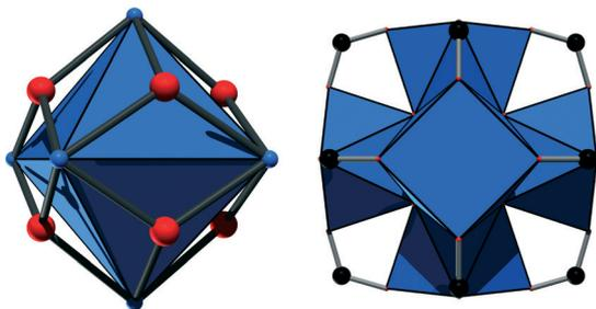
**Fig. 1** Left: representation of the  $Zr_6$  octahedron with face-capping oxygen atoms. Zirconium atoms are in blue and oxygen atoms are in red. Right: complete inorganic node including carboxylate groups, as it is observed in the UiO-66 structure. ZrO polyhedra are in blue and carbon atoms are in black.
