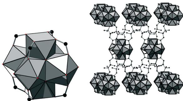
Fig. 3 The eight-connected inorganic node is shown on the left. On the right, the framework connectivity (bcu topology) is illustrated, showing a  $2 \times 1 \times 1$  supercell. Carbon atoms are shown in black and ZrO polyhedra in grey.
