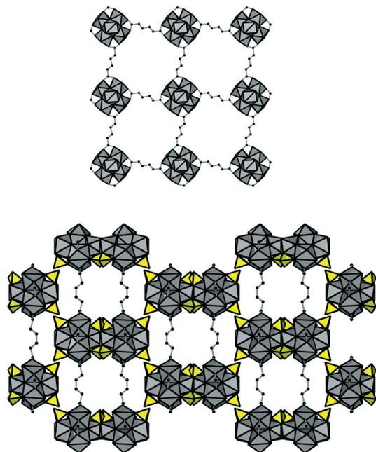
Fig. 5 Top: the square grid layer in 2 formed by the interconnection of inorganic nodes *via* adipate molecules, as seen along the *c*-axis. Bottom: the framework structure of 2 as seen along the *a*-axis. Guest molecules filling the channels are omitted for clarity. ZrO polyhedra are shown in grey, sulfate ions in yellow and carbon atoms in black.
