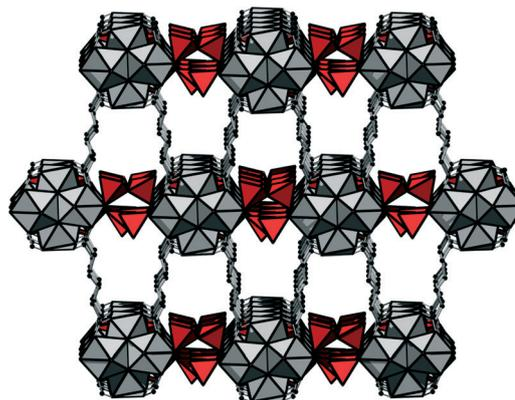
Fig. 7 Framework structure of **3** as seen along [110]. Guest molecules present inside the cavities are omitted for clarity. ZrO polyhedra are shown in grey,  $\text{Cr}_2\text{O}_7^{2-}$  ions in red and carbon atoms in black.
