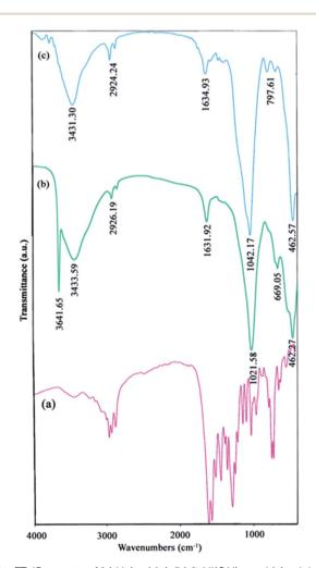
Fig. 1 FT-IR spectra of (a)  $H_2(pnAA_2)$ , (b)  $\beta$ -Ni(OH)<sub>2</sub>, and (c) calcinated NiO at 750 °C.
