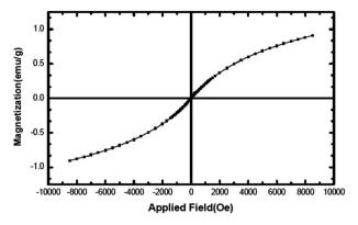
Fig. 6 Magnetization *versus* applied magnetic field at room temperature for NiO nanoparticles.
