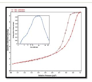
Fig. 7  $N_2$  adsorption—desorption isotherm and pore size distribution (inset) of NiO nanoparticles.
