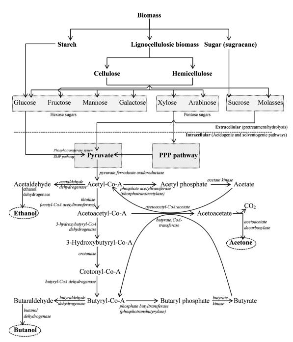
Fig. 1 The metabolic pathway of acetone-butanol-ethanol (ABE) fermentation by C. acetobutylicum.<sup>23,41,116</sup>
