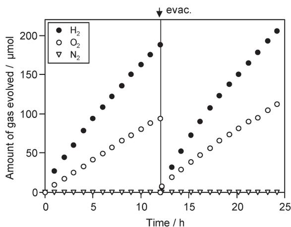
**Fig. 2** Time course of photocatalytic evolution of H<sub>2</sub> and O<sub>2</sub> using a mixture of Pt (0.3 wt%)–TaON (0.2 g) and Pt (0.5 wt%)–WO<sub>3</sub> (0.2 g) suspended in a 5 mM NaI aqueous solution (pH 7 without adjustment) under visible light ( $\lambda > 420$  nm).
