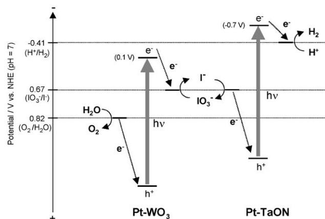
**Fig. 3** Speculated reaction mechanism for water splitting over Pt–TaON and Pt–WO<sub>3</sub> with an  $\text{IO}_3^-/\text{I}^-$  shuttle redox mediator.
