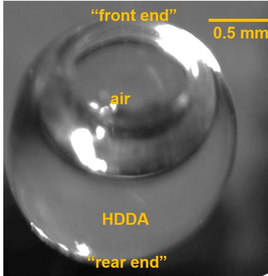
FIG. 6: Image of a HDDA-coated bubble after polymerization.
