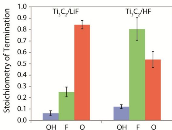
Figure 3: Composition of the  $\text{Ti}_3\text{C}_2\text{T}_x$  surface functional groups produced by etching of the  $\text{Ti}_3\text{AlC}_2$  in HF and LiF-HCl solutions, per  $\text{Ti}_3\text{C}_2$  formula unit, i.e.  $\text{Ti}_3\text{C}_2(\text{OH})_x\text{F}_y\text{O}_z$ .
