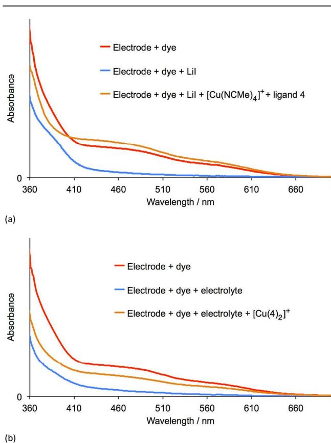
Fig. 9. Solid-state absorption spectra of transparent electrodes (no scattering layer on the  $\text{TiO}_2$ ) functionalized with the dye  $[\text{Cu}(\mathbf{1})(\mathbf{4})]^+$  (red) and post-treated (a) with Lil solution (blue), then  $[\text{Cu}(\text{NCMe})_4][\text{PF}_6]$  followed by ligand  $\mathbf{4}$  (orange), and (b) with  $\text{I}^-/\text{I}_3^-$  electrolyte (blue), then  $[\text{Cu}(\mathbf{4})_2]^+$ .
