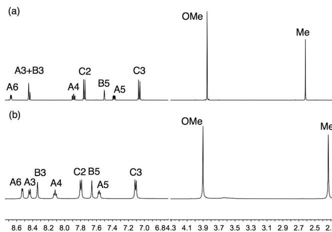
Fig. 1. 500 MHz NMR spectra of (a) ligand **5** in  $\text{CD}_3\text{CN}$ , and (b)  $[\text{Cu}(\mathbf{5})_2][\text{PF}_6]$  in  $\text{CD}_2\text{Cl}_2$  ( $\approx 295$  K). For atom labelling, see Scheme 2. A common solvent could not be used for ligand and complex.
