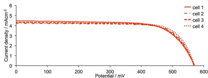
Fig. 5.  $J-V$  curves for sets of four DSCs containing the dyes  $[\text{Cu}(\mathbf{2})(\mathbf{6})]^+$  measured on the day of cell assembly to confirm performance reproducibility. Analogous sets of data for DSCs containing the dyes  $[\text{Cu}(\mathbf{2})(\mathbf{3})]^+$ ,  $[\text{Cu}(\mathbf{2})(\mathbf{4})]^+$  and  $[\text{Cu}(\mathbf{2})(\mathbf{5})]^+$  are shown in Fig. S1<sup>†</sup>.
