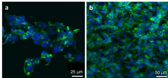
**Fig. 7** Confocal microscopy images of the extracted hydrogel constructed in a (a) nutrient-poor environment (0% medium concentration) at nodal location 1 (see Fig. 1(a)), and, (b) nutrient-rich environment (100% medium concentration) at nodal location 5. The cell nuclei stained by DAPI is shown in blue whereas cell F-actin networks stained by phalloidin are displayed in green.
