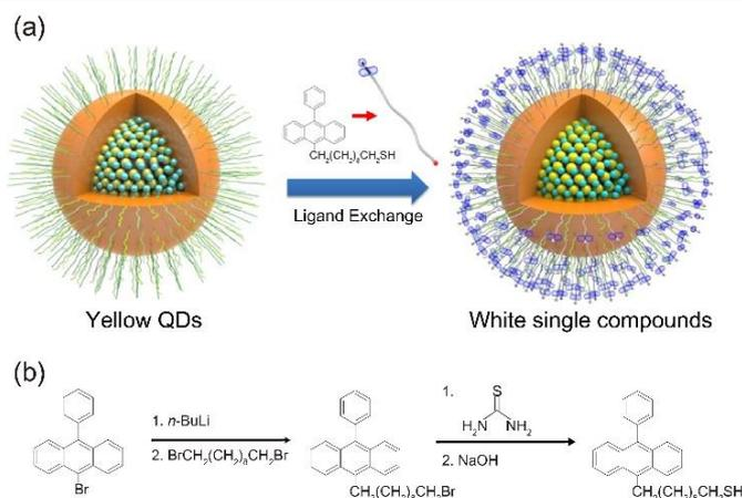
**Scheme 1.** (a) Schematic illustration of preparation of white-light emitting quantum dot of single compound through ligand exchange and (b) scheme for the synthesis of thiol-containing long alkyl chain anthracene ligands(PADT).
