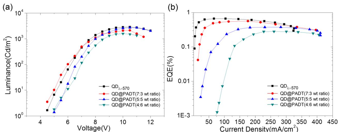
Figure 4. (a) Luminance-voltage (L-V) curves for the QD-WLED devices (b) External quantum efficiency-current density (EQE-J) curves for the devices.
