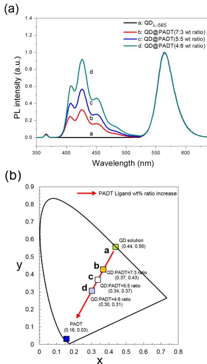
**Figure 2.** (a) Emission spectra ( $\lambda_{ex}=365\text{nm}$ ) of CdSe/ZnS QDs with variable weight ratio of QD to PADT (b) CIE 1931 chromaticity diagram. The color square shows the luminescent color coordinates for the corresponding states a(0.44, 0.56), b(0.37, 0.43), c(0.34, 0.37), d(0.30, 0.31) and PADT(0.16, 0.03), respectively.
