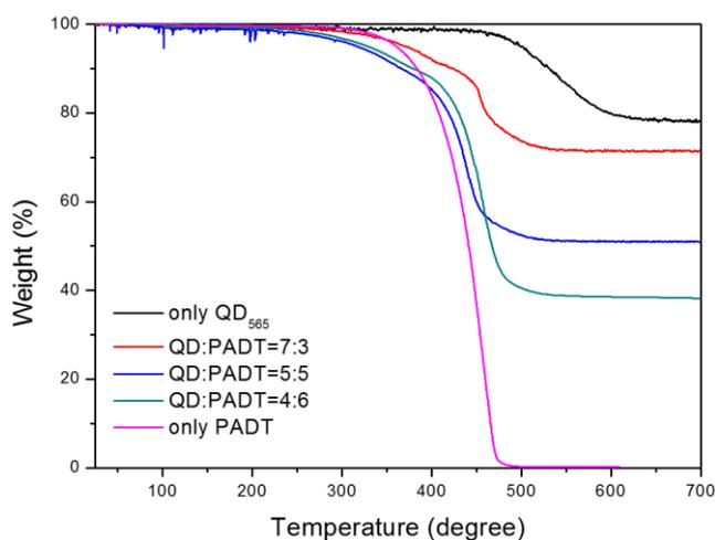
**Figure 1.** Thermal gravimetric analysis of pristine QDs, PADT, and different weight ratio of single compound.
