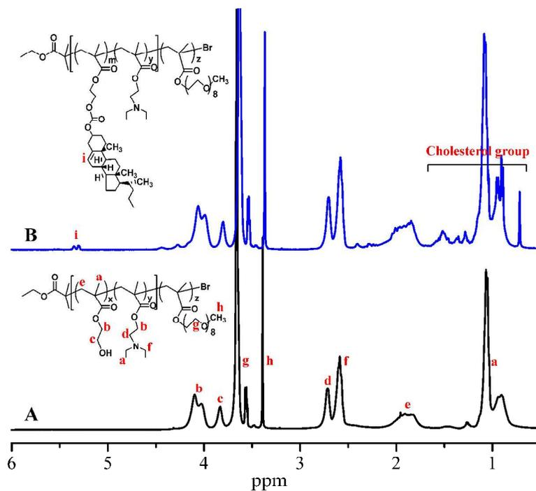
Fig. 2  $^1\text{H}$  NMR spectra of P(HEMA<sub>10</sub>-*co*-DEA<sub>25</sub>)-*b*-PPEGMA<sub>10</sub> (A) and Chol-P(HEMA<sub>10</sub>-*co*-DEA<sub>25</sub>)-*b*-PPEGMA<sub>10</sub> (B) in *d*-CDCl<sub>3</sub>
