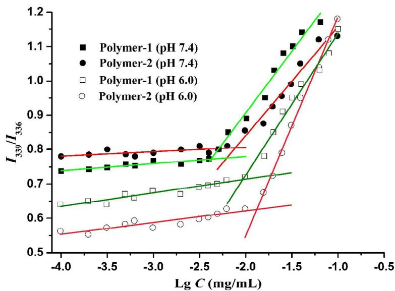
Fig. 3 pH-dependent CMC of micelle self-assembled from polymer-1 and polymer-2.
