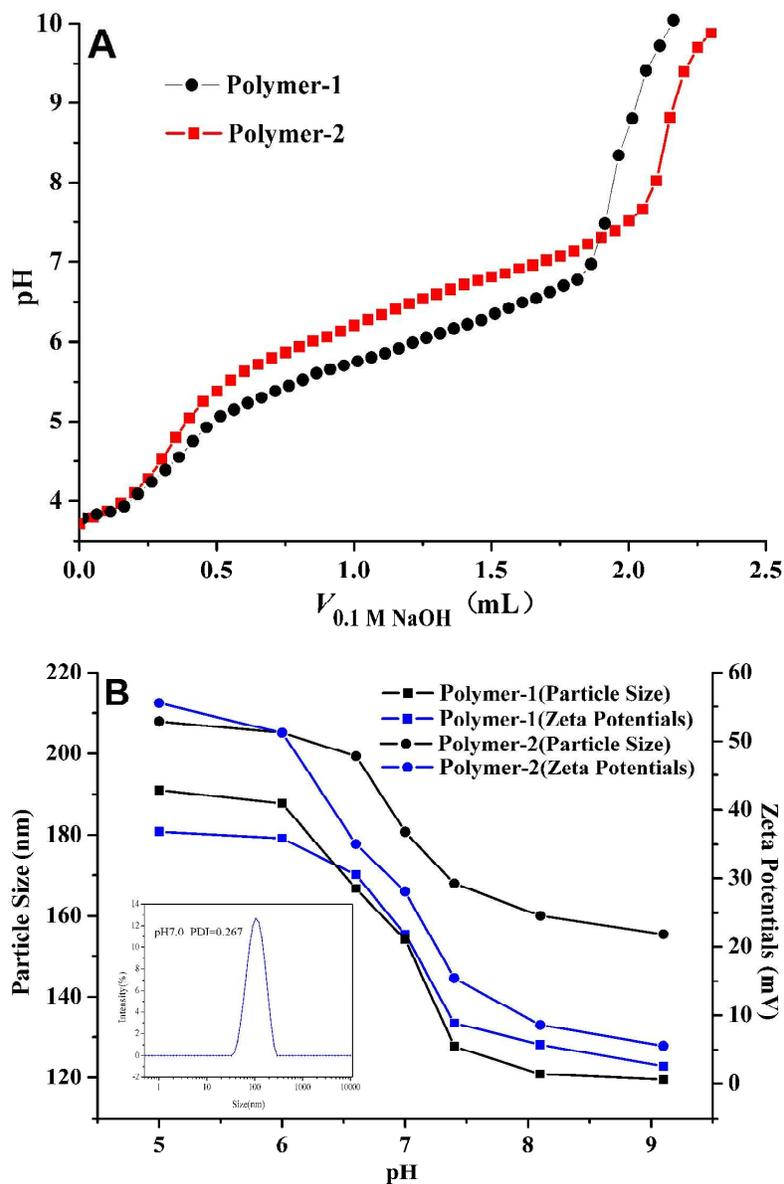
Fig. 4 Titration curves of two synthesized copolymers (A), micelle size and zeta potentials (B) of polymeric micelles as a function of pH
