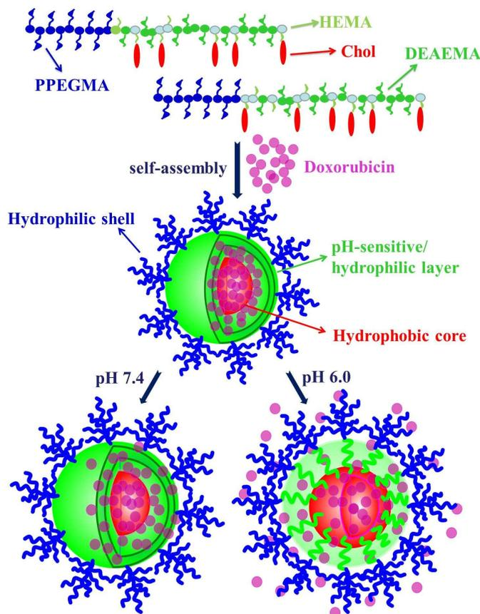
Scheme 1. Scheme of drug entrapment and pH-dependent release from the polymeric micelles
