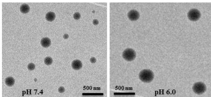
Fig. 5 Typical TEM images of micelles in different PBS buffer solutions.
