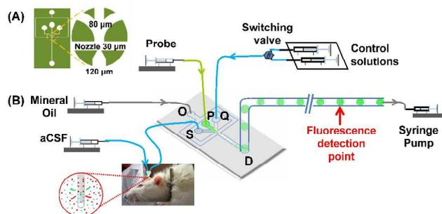
**Scheme 1.** (A) CAD design of the droplet-formation microfluidic chip; (B) Illustration of the integrated microdialysis/droplet-based microfluidic chip system for in-vivo measurement of the HS<sup>-</sup> concentration in rat's brain.
