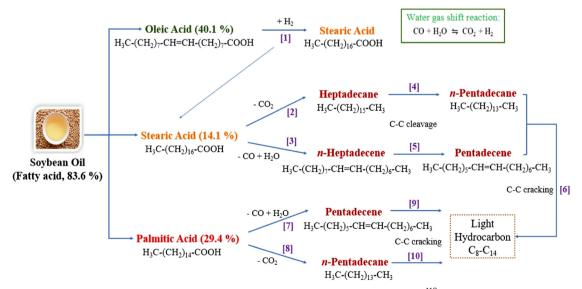
Fig. 4 Proposed catalytic deoxygenation reaction mechanism of soybean oil using an NiO-CD catalyst. 118
