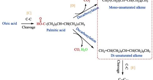
Fig. 3 Proposed deoxygenation reaction pathway for the deoxygenation of WCO to hydrocarbon over CaO-La<sub>2</sub>O<sub>3</sub>/AC catalysts.
