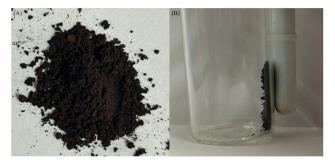
Fig. 6 Images of (A) the prepared Fe<sub>3</sub>O<sub>4</sub> catalyst and (B) Fe<sub>3</sub>O<sub>4</sub> catalyst attracted to a magnetic bar.
