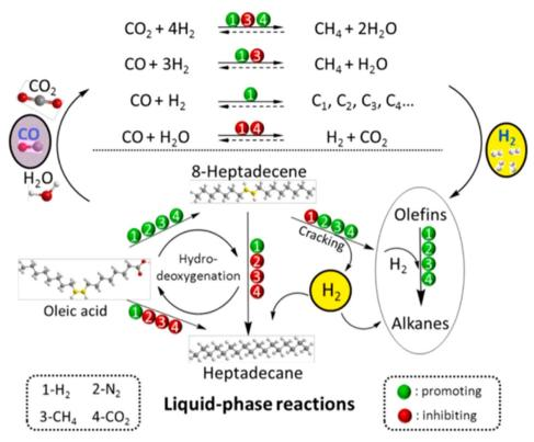
Fig. 8 Impact of four distinct reaction gasses on the reaction route that leads to the deoxygenation of oleic acid. This reference is protected by copyright.419
