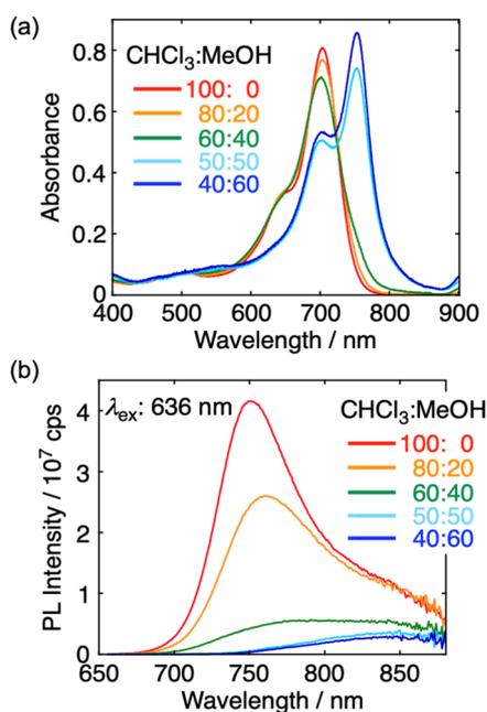
Fig. 2 (a) UV-vis-NIR absorption spectra and (b) fluorescence spectra of **TACIC-Br** in a mixture of  $\text{CHCl}_3$  and MeOH ( $1 \times 10^{-5}$  M). The inset depicts the ratio of  $\text{CHCl}_3$ : MeOH (v/v).
