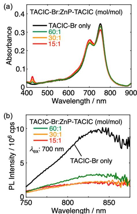
Fig. 6 (a) UV-vis-NIR absorption spectra and (b) fluorescence spectra of TACIC-Br/ZnP-TACIC in a mixture of CHCl<sub>3</sub> and MeOH ( $1 \times 10^{-5}$  M, 50 : 50, v/v). The inset depicts the molar ratio of TACIC-Br : ZnP-TACIC.
