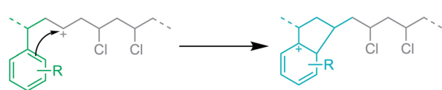
Fig. 2 Proposed intramolecular Friedel–Crafts alkylation leading to formation of polyindene segments.
