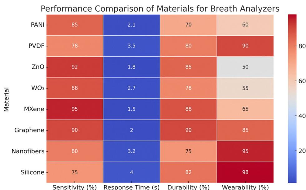
Fig. 17 Performance comparison of materials for breath analyzers.
