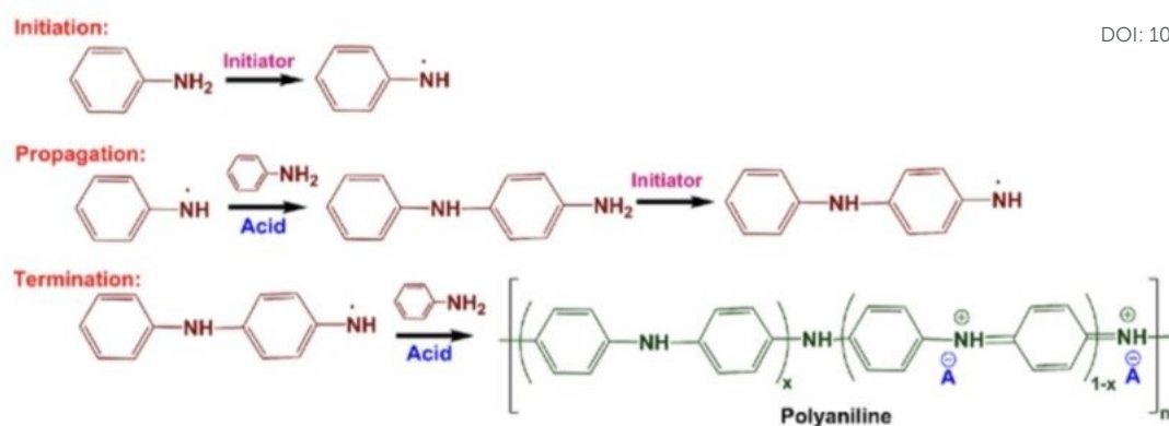
Figure 4 Chemical polymerization mechanisms of polyaniline. Chemical polymerization of polyaniline is carried out in acidic medium by using a common initiator such as ammonium persulfate and potassium persulfate. 99 Reproduced with permission from ACS.
