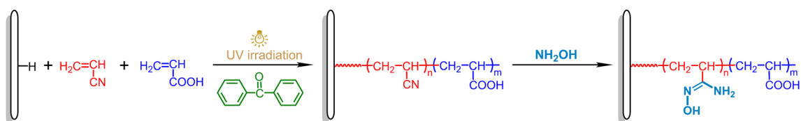
Scheme 1 Schematic diagram for the synthesis of amidoxime MBF adsorbents.
