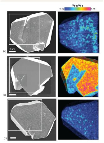
Fig. 5 Morphological characteristics shown by SEM and correlative NanoSIMS isotopic mapping on the (a) control NAFe(II)-oxalatehematite, (b) <sup>57</sup>Fe(II)-hematite, (c) <sup>57</sup>Fe(II)-oxalate-hematite samples.
