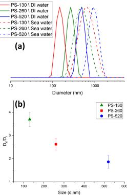
**Fig. 5** Comparing (a) size distribution by intensity of DLS analysis for PS particles in DI water *versus* seawater and (b) particle size ratio of them ( $D_s$  and  $D_i$  are the particle size respectively in sea water and DI water.)
