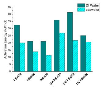
Fig. 7 Activation energy  $(E_a)$  of  $Cu^{2+}$  adsorption by original and UVaged PS particles in DI water and seawater.
