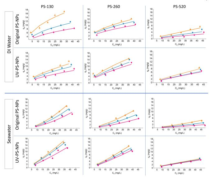
Fig. 8 The effect of temperature on the  $Cu^{2+}$  adsorption isotherms by different size ranges of original and UV-aged PS-NPs in DI water and seawater (290 K  $_{\triangle}$ , 300 K  $_{\square}$ , 310 K  $_{\square}$ ).
