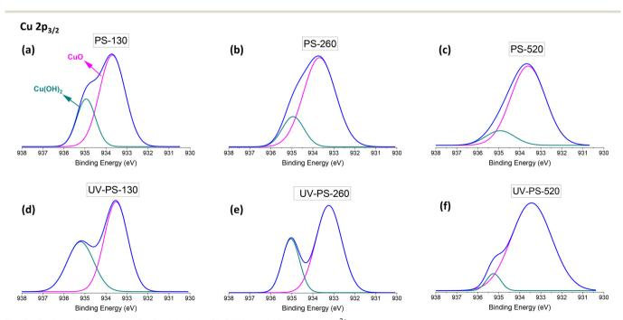
Fig. 6 Cu 2p<sub>3/2</sub> XPS spectra of (a-c) original and (d-f) UV-aged PS-NPs after Cu<sup>2+</sup> adsorption.
