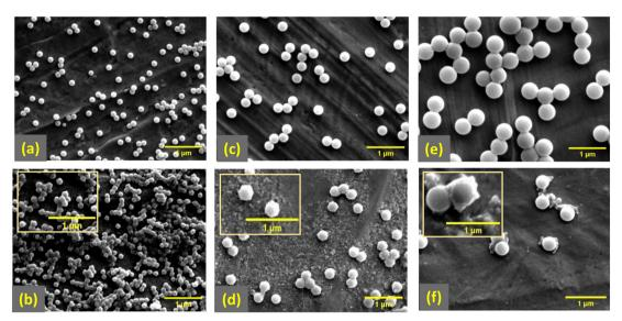
Fig. 2 SEM images of (a and b) PS-130, (c and d) PS-260 and (e and f) PS-520 in their original and UV-aged forms, respectively.
