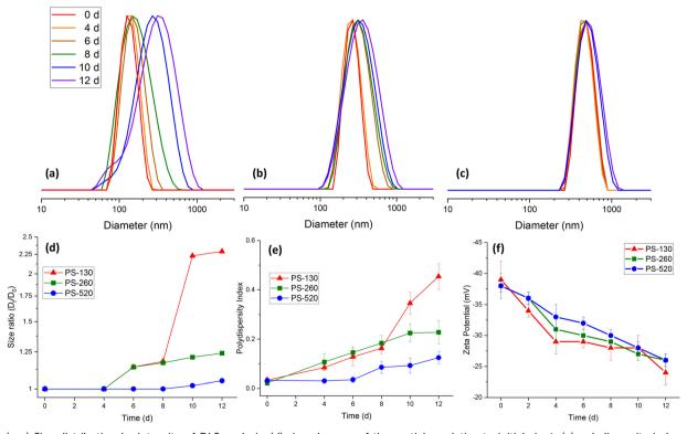
Fig. 1 (a-c) Size distribution by intensity of DLS analysis, (d) size changes of the particles relative to initial size\*, (e) polydispersity index of DLS analysis and (f) zeta potential of the particles at different time intervals during UV-degradation. Error bars represent the standard deviations. \*Do and  $D_t$  represent initial diameter and the diameter at time t, respectively.
