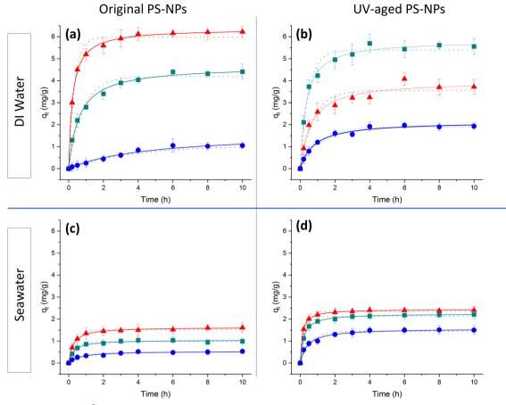
Fig. 4 Adsorption kinetics of  $Cu^{2+}$  in (a and b) DI water and (c and d) seawater for original and UV-aged PS-130 ( $\triangle$ ), PS-260 ( $\blacksquare$ ) and PS-520 ( $\bigcirc$ ), including PFO (dotted line) and PSO (solid line) model fittings.
