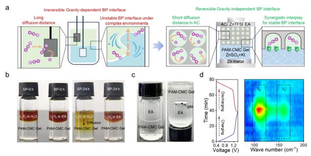
Fig. 6 (a) The design of gravity-dependent and gravity-independent BP interfaces. (b) The photos for the shuttle experiment of I<sub>3</sub><sup>-</sup>/I<sub>2</sub> in EA/PAM-CMC (BP) and H<sub>2</sub>O/PAM-CMC (SP) systems. (c) The photos of gravity-independent test of EA/PAM-CMC. (d) The in situ Raman spectra of Zn-iodine based on the BP electrolyte during the charging/discharging process.
