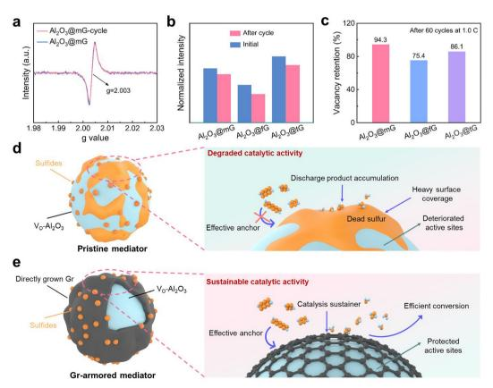
Fig. 3 Mechanism of active site failure and protection. (a) Ex situ EPR spectra of Al<sub>2</sub>O<sub>3</sub>@mG. (b) EPR intensity of different Al<sub>2</sub>O<sub>3</sub>@G samples before and after cycling. (c) Corresponding vacancy retention rates after 60 cycles at 1.0 C. Schematic illustrating the evolution of vacancy sites on (d) the pristine mediator and (e) the graphene-armored mediator during the electrochemical process.
