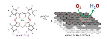
Multihalogenated Zn phthalocyanine as a precursor for porous Zn-N<sub>4</sub>-C carbons toward electrocatalytic oxygen reduction
