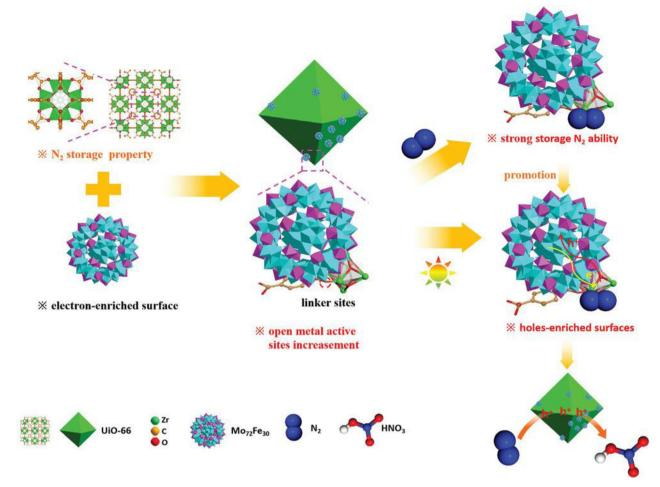
Fig. 7 Schematic illustration of the efficient storage and conversion of  $N_2$  to  $HNO_3$  by POM@MOF (taking UiO-66 and  $Mo_{72}Fe_{30}$  as an example). Reproduced from ref. 38 with permission from John Wiley and Sons, copyright 2023.
