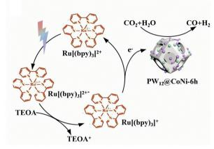
Fig. 4 (a) Schematic presentation of the band positions of  $Cu_x[POM]@-$ TiO<sub>2</sub> along with photochemical CO<sub>2</sub> reduction scheme in the presence of 390 nm LED lamp. 86 Reproduced from ref. 86 with permission from John Wiley and Sons, copyright 2024. (b) PW<sub>12</sub>@CoNi in photosensitizer system CO<sub>2</sub> reduction mechanism diagram.<sup>89</sup> Reproduced from ref. 89 with permission from Elsevier, copyright 2024.
