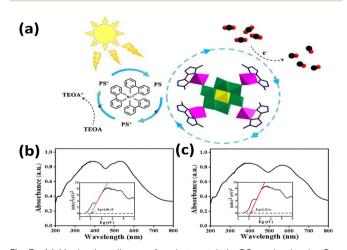
Fig. 3 (a) Mechanism diagram for photocatalytic CO<sub>2</sub> reduction by Co-CrMo<sub>6</sub>. (b) UV-vis diffuse reflection spectra and K-M function curve of Co-CrMo<sub>6</sub>. (c) UV-vis diffuse reflection spectra and K-M function curve of Zn-CrMo<sub>6</sub>.<sup>79</sup> Reproduced from ref. 79 with permission from American Chemical Society, copyright 2022.
