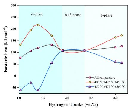
Fig. 5 Isosteric heat of hydrogen absorption ( $Q_{st}$ ) as a function of hydrogen uptake for the LiH-PSiNW alloy at different temperature zones.
