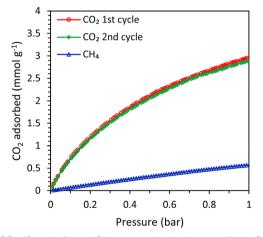
Fig. 7 CO<sub>2</sub> (2 cycles) and CH<sub>4</sub> adsorption isotherms of the SAPO-34 beads
