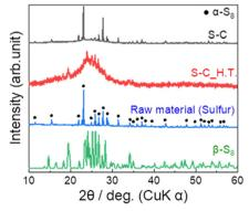
Fig. 2 The XRD patterns of the prepared S-C and S-C\_H.T. For comparison, the XRD patterns of the raw material  $\alpha$ -sulphur (black circles  $\bullet$ ) and **β**-sulphur are also shown
