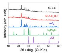
Fig. 6 The XRD patterns of SE-S-C and SE-S-C\_H.T. For comparison, the XRD patterns of  $\alpha$ -sulphur, Li<sub>6</sub>PS<sub>5</sub>Cl, and LiCl are also provided. The inverted triangle  $(\nabla)$  indicates the observed small peak at around 30°
