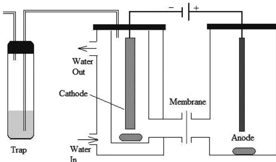
Fig. 11 Electrochemical hydrogenation cell setup for ECH of water-soluble bio-oil.<sup>72</sup>
