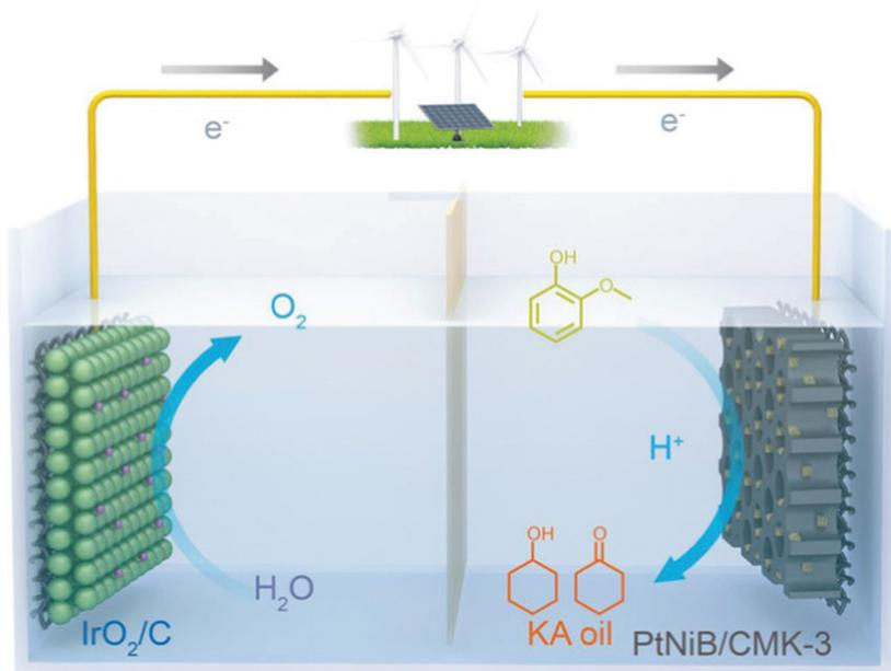
Fig. 7 Schematic of ECH of guaiacol into KA oil integrated with  $O_2$  production, equipped with PtNiB/CMK-3 and  $IrO_2/C$  as the cathode and anode, respectively. Reprinted with permission from ref. 42 Copyright 2019 Wiley.
