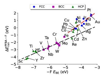
Fig. 6  $\Delta E_{rxn}^{PFBA-F}$  vs. fluorine binding for the removal of a -F from a  $C_{\alpha}$ carbon on transition metal surfaces. The black dashed line represents a linear fit to the data for the carbo binding mode ( $\Delta E_{rxn}^{PFBA-F} = 0.95E^{-}$  $^{F}_{BE}$  + 3.09,  $R^2$  = 0.92). The red dashed line represents a linear fit to the flat binding mode ( $\Delta E_{TXN}^{PFBA-F}$  = 1.59 $E_{BE}^{-F}$  + 6.98,  $R^2$  = 0.67).
