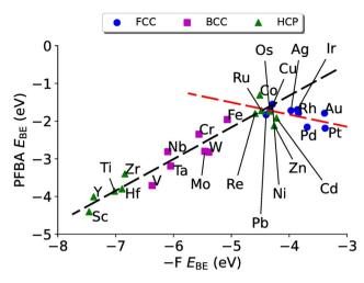
Fig. 4 PFBA binding vs. fluorine binding on transition metal surfaces. The black dashed line represents a linear fit to the data for the carbo binding mode ( $E_{\rm BE}^{\rm PFBA}=0.84E_{\rm BE}^{\rm FF}+2.04$ ,  $R^2=0.91$ ). The red dashed line represents a linear fit to the flat binding mode ( $E_{\rm BE}^{\rm PFBA}=-0.32E_{\rm BE}^{\rm F}-3.12$ ,  $R^2=0.27$ ).
