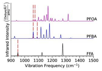
Fig. 3 Calculated infrared vibrational spectra for FFA, PFBA, and PFOA in the gas-phase. The red dashed vertical lines denote locations of the C-F stretch (FFA) and the location of the  $-C_{\alpha}F_2$ - stretches (PFBA and PFOA). Numerical data and mode assignments are in Tables S8-S10.†
