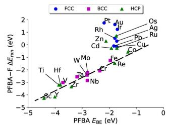
Fig. 5 PFBA binding vs.  $\Delta E_{rxn}^{PFBA-F}$  for the removal of a -F from a  $C_{\infty}$  carbon on transition metal surfaces. The black dashed line represents a linear fit to the data for the carbo binding mode ( $\Delta E_{rxn}^{PFBA-F} = 0.57E_{BE}^{PFBA} + 1.06$ ,  $R^2 = 0.90$ ). No stable solution exists for the linear regression of the flat binding mode.
