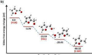
Fig. 8 (a) In situ ATR-IR spectra of furfural (FUR) conversion to 2-methylfuran (2-MF) with furfuryl alcohol (FAL) as an intermediate at 60 °C for 90 min in i-PrOH at regular intervals of 30 min and (b) energy profile diagram of catalytic conversion of furfural (FUR) to 2-methylfuran (2-MF).
