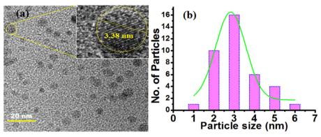
Fig. 2 (a) TEM images and inset is the magnified image of HRTEM and (b) the size distribution histogram of OCDs
