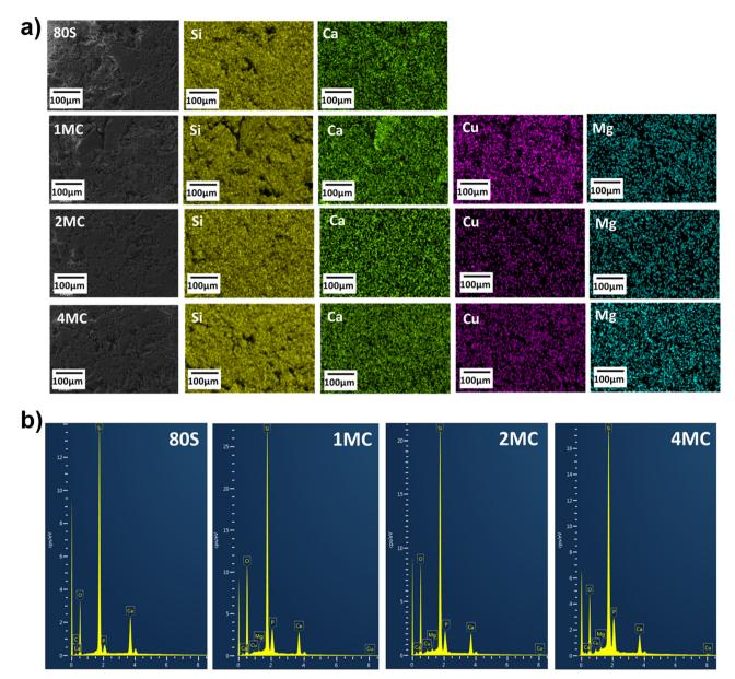
Fig. 3 Lateral SEM-EDX mapping of co-doped mesoporous glass powders (a); EDX spectra (b) measured during mapping
