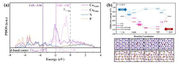
Fig. 5 DTF calculation for CoP/CoN@NCNRs/CC: (a) PDOS calculation, and (b) free energy plot for the ORR and OER on CoN, CoP and CoP/ CoN; reaction mechanisms for the OER and ORR on the target-specific N side and P side, respectively
