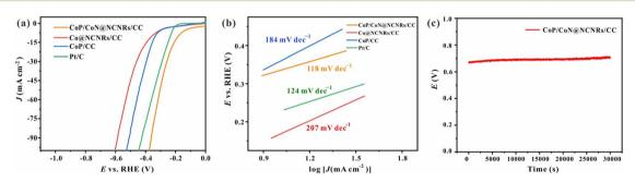
Fig. 6 Electrochemical testing of the HER and OER: (a) LSV curve of the HER, (b) Tafel slope of the HER, and (c) the chronoamperometric response of the HER.
