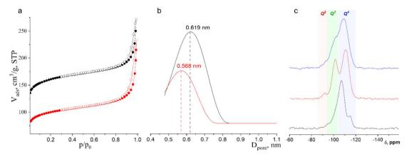
Fig. 4 (a) Argon adsorption/desorption isotherms for parent IWR and daughter IPC-17 zeolites; (b) pore size distribution of parent IWR (black) and daughter IPC-17 zeolites (red); and (c) <sup>29</sup>Si MAS NMR spectra of initial IWR (black), intermediate IPC-17P (red), and IPC-17 (blue) samples.
