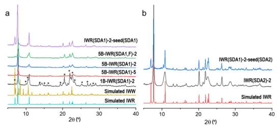
Fig. 1 (a) XRD patterns of IWR samples prepared from reaction mixtures with variable B content and Si/Ge molar ratios in the presence of SDA1. Characteristic diffraction lines of the IWW zeolite admixture in the 1B-IWR(SDA1)-2 sample are marked by asterisks. (b) XRD patterns of IWR samples prepared from B-free reaction mixtures with a Si/Ge molar ratio of 2 using different SDAs.
