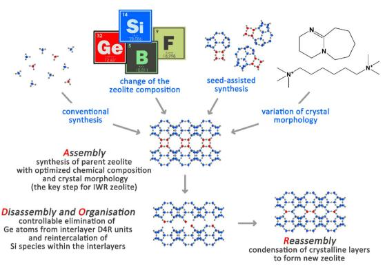
Scheme 1 Schematic representation of the ADOR steps for the IWR zeolite under study. Ge atoms participating in the formation of D4R units inbetween the crystalline silica layers are highlighted in red, while Si atoms are highlighted in blue.
