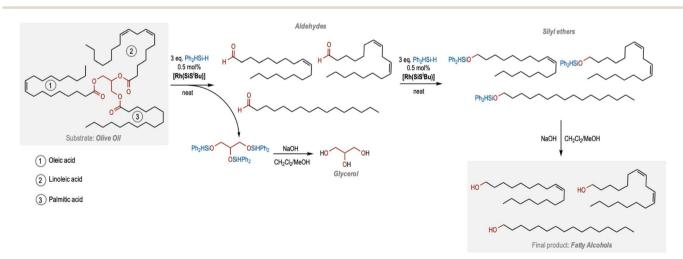
Fig. 2 Proposed pathway to produce fatty alcohols from plant oils.
