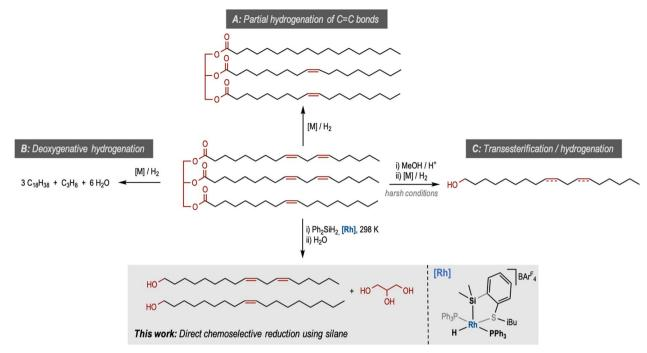
Different pathways for the reduction of plant oils and the structure of the [Rh(SiSiBu)] complex used in this study
