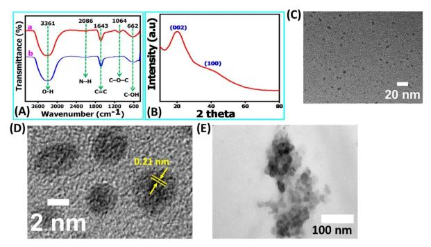
Fig. 2 Characterization and morphological analysis of NR-CDs and their interaction with Fe<sup>2+</sup> ions. (A) FT-IR spectra of neem resign extracts (dark red line) and the NR-CDs (dark blue line). (B) XRD pattern and (C and D) TEM image of the NR-CDs. (E) TEM image of NR-CDs in the presence of 62  $\mu$ M of Fe<sup>2+</sup> ions.
