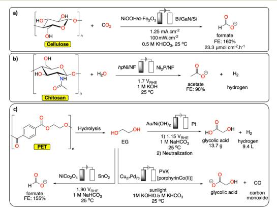
Fig. 13 Parallel paired electrolysis polymer recycling methodologies. (a) Electrochemical conversion of cellulose/CO<sub>2</sub> to formate;<sup>106</sup> (b) electrochemical chitosan to acetate conversion with concomitant hydrogen production;107 (c) electrochemical conversion of EG/CO<sub>2</sub> to various products.16,108-110
