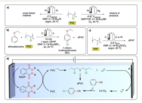
Fig. 9 Electrochemical dehalogenation. (a) Electrochemical degradation of PVC; (b) tandem electrochemical dechlorination of PVC with concomitant chlorination of an electron-rich arene;85 (c) electrochemical defluorination of PVF;89 (d) schematic representation of the DEHPmediated reductive dichlorination of PVC coupled with chlorination of an electron-rich arene. The abbreviations dPVC and dPVF refer to (partial) dechlorinated PVC and (partial) defluorinated PVF, respectively.85
