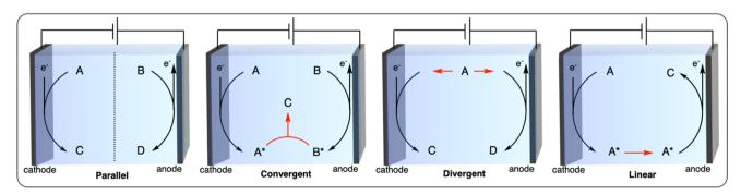
Fig. 12 Schematic representation of the most common paired-electrolysis reactions
