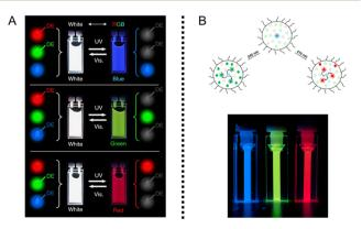
Fig. 5 (A) The photoswitching fluorescence of a mixed solution based on the combination of three distinct types of PF NPs.<sup>40</sup> Adapted with permission from ref. 37. Copyright 2014 Springer Nature. (B) Scheme of multiple-emission in single PF NPs.<sup>97</sup> Adapted with permission from ref. 92. Copyright 2019 Springer Nature.
