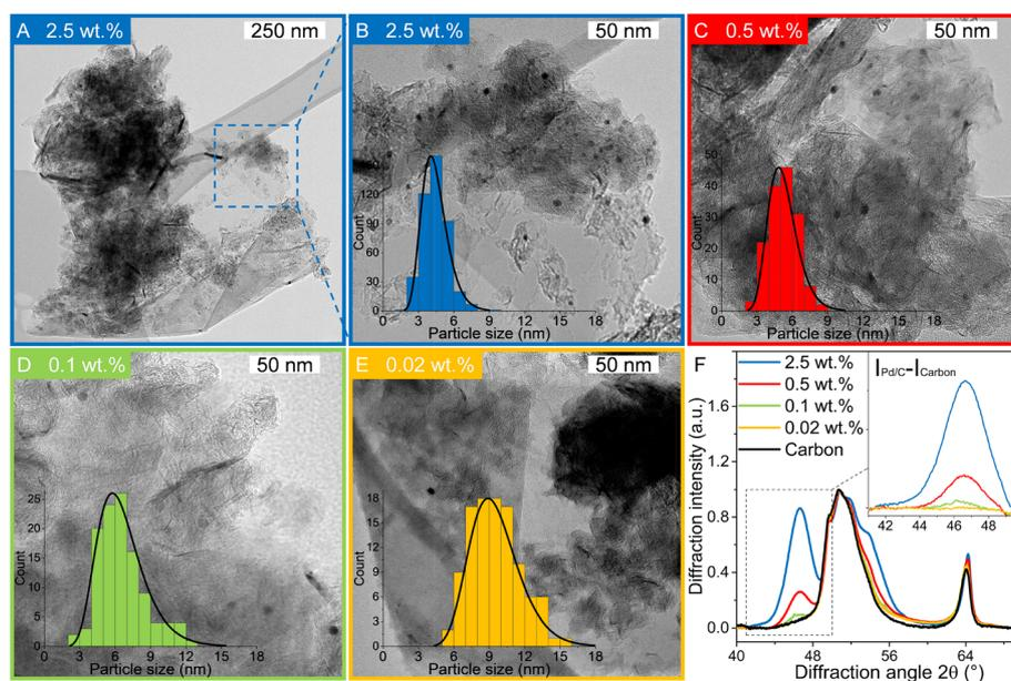
**Fig. 2** Catalyst characterisation. (A–E) Transmission Electron Microscopy (TEM) images of Pd/C catalysts with Pd weight loading of (A) 2.5 wt% (low) and high (B) magnification, (C) 0.5 wt% (D) 0.1 wt% and (E) 0.02 wt%. Insets shown size histograms of the individually measured diameters from TEM and lognormal fit to the distribution. (F) X-ray diffractogram of the Pd/C catalysts. The inset shows the carbon-subtracted intensity, highlighting the Pd(111) diffraction at 46.6° 2θ.
