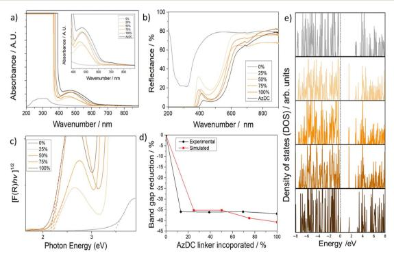
Fig. 5 (a) Solid-state UV-vis profiles of the samples. (b) Reflectance profiles of the samples. (c) Tauc plots of the samples. (d) Comparison of the percentage of decrease in experimental and calculated band gap values of the MTV MOFs upon the introduction of AzDC. (e) Total projected density of states of the MTV series
